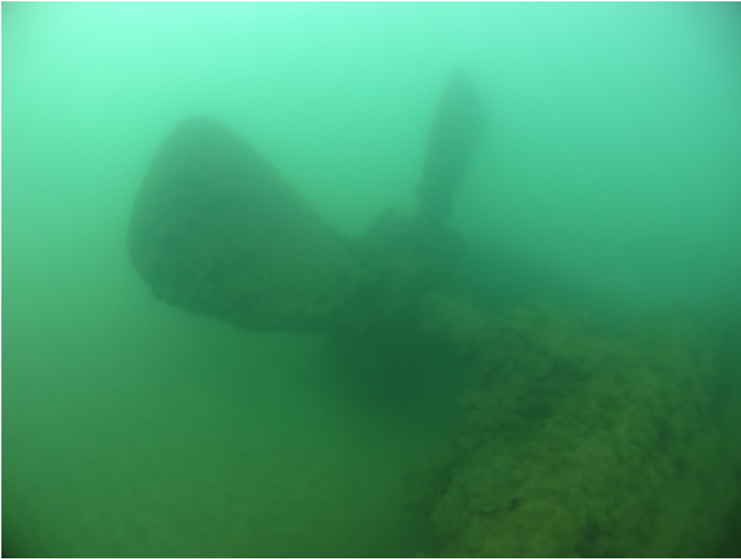
Figure 6 Propeller of the Muskegon remains intact and good condition but is covered in invasive zebra mussels.
