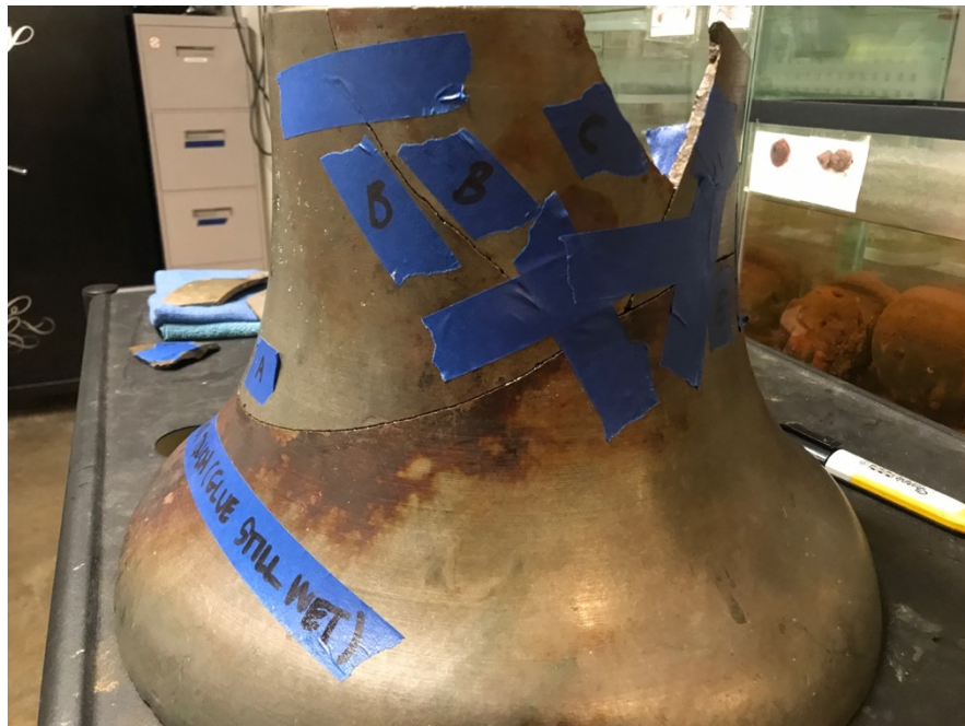
Figure 4. The bell, mid-conservation, with masking tape to ensure that pieces do not move during the curing process.
