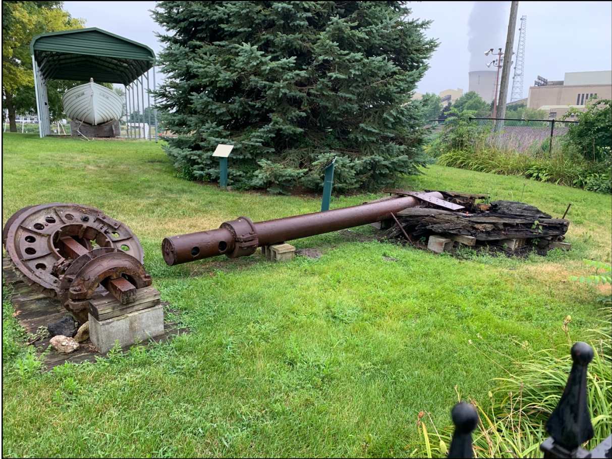
Figure 3. The J.D. Marshall's rudder assembly and deck winch.
